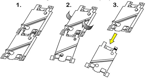
The following 3 sketches show how to assemble the 'track plate'.
