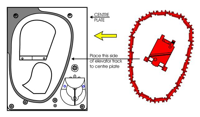
2. Once the 'track plate' is in position, turn the track through 720 to ensure it is seated in the guide path correctly.
