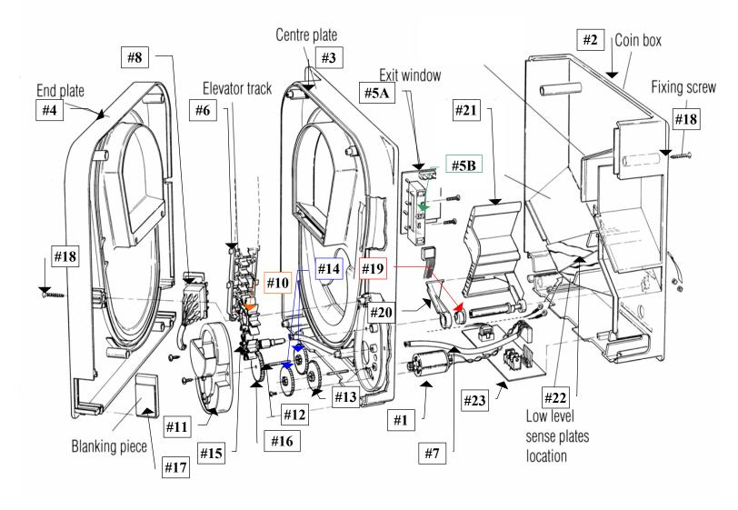
**#17** - 1040-24-22 Blanking Plate **#18** - 1040-24-25 Fixing screw #19 - 1041-24-19 Cam Shaft 1041-24-20 Cam shaft bearing
